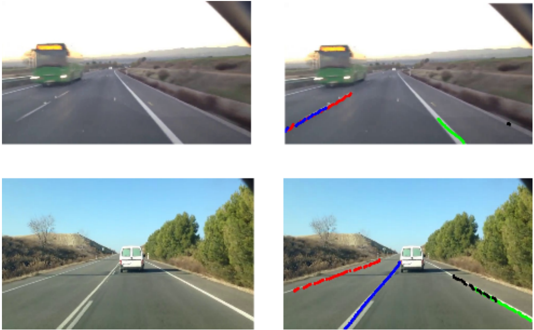
Figure 3.15: Poor Results from SCNN
