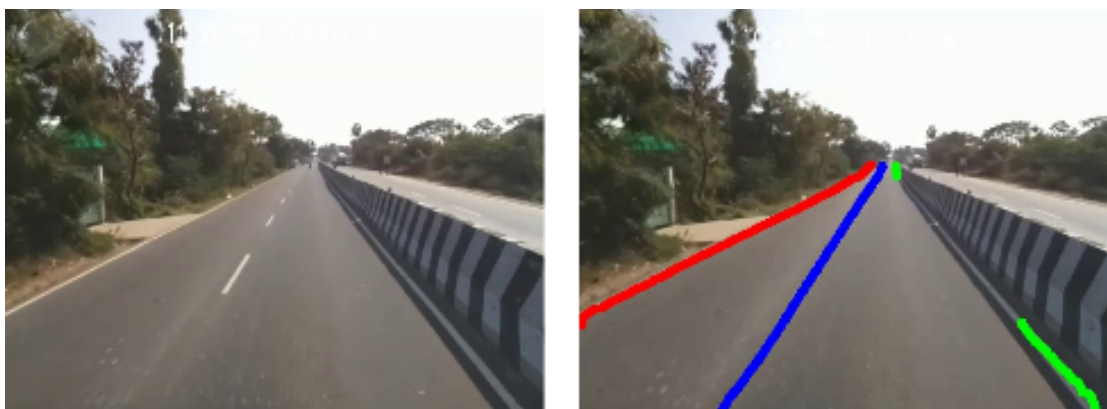
Figure 3.14: SCNN Result for Lanes Under Shadow
