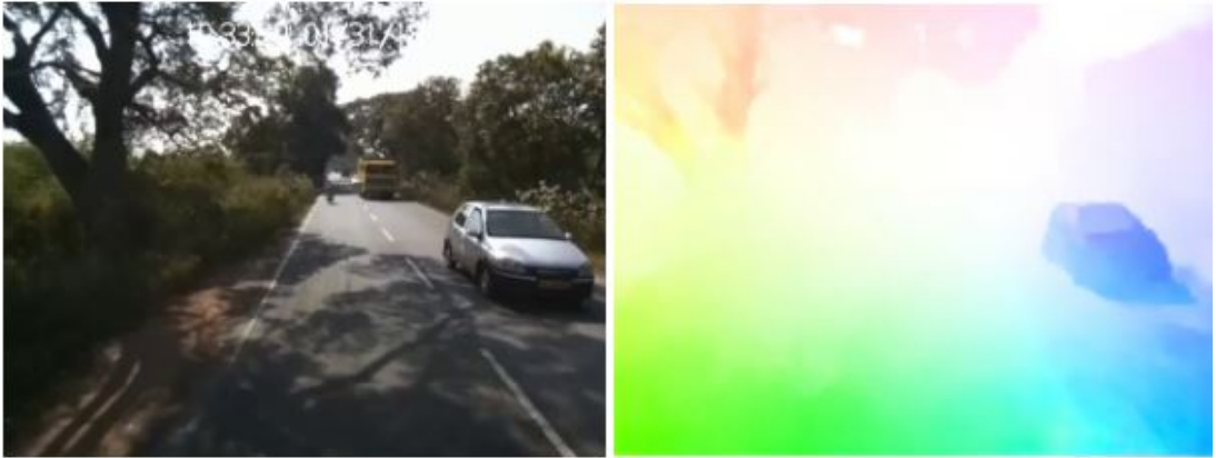
Figure 3.20: Sample Frame and its Optical Flow Output from PWC-Net
