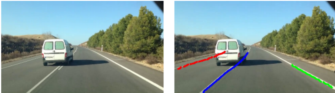
Figure 3.13: SCNN Result for Partially Occluded Lanes
